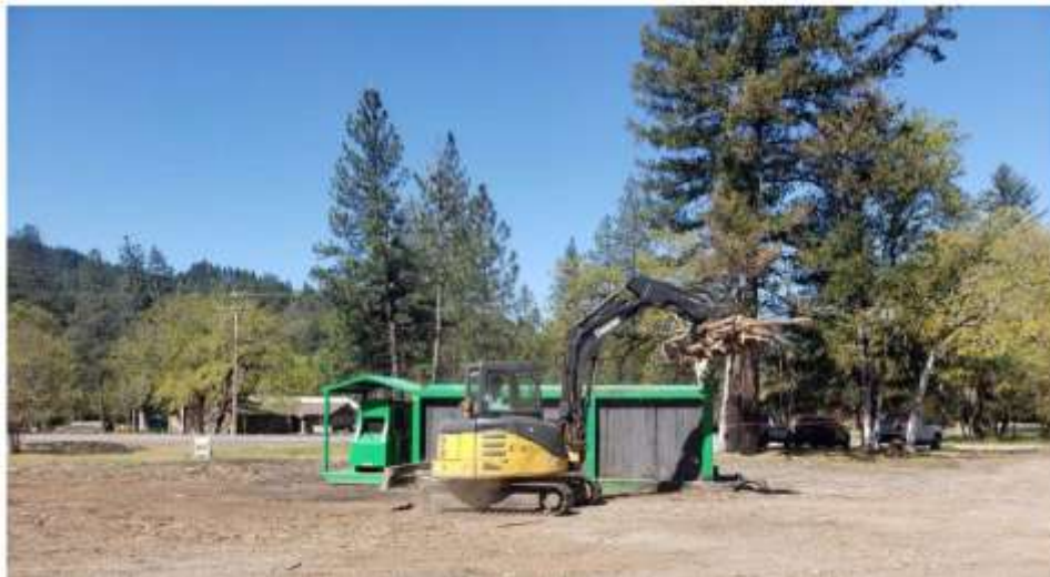
Figure 9. Six Rivers National Forests' dozer operator adds woody debris into CAL FIRE's air curtain burner, utilized for fuels reduction throughout the Mad River Ranger District.
