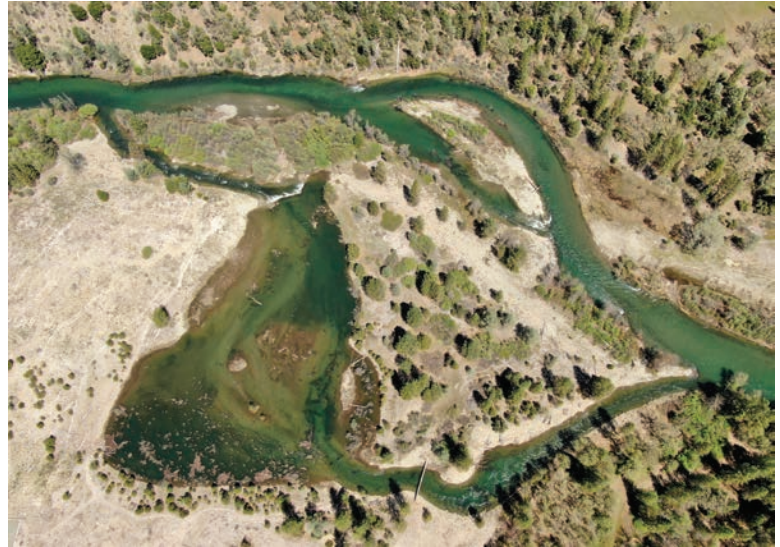
This image shows the Bucktail channel rehabilitation site in April 2019, three years after construction. The Bucktail channel rehabilitation site was designed to build and sustain dynamic mainstem bar (point, medial) and riffle morphology, and off-channel rearing areas designed to increase and sustain the availability, quantity, and quality of anadromous fish habitat between 300 cfs and 2,000 cfs for all life stages. Photo by A. Martin, Yurok Tribal Fisheries Dept., 2019.
